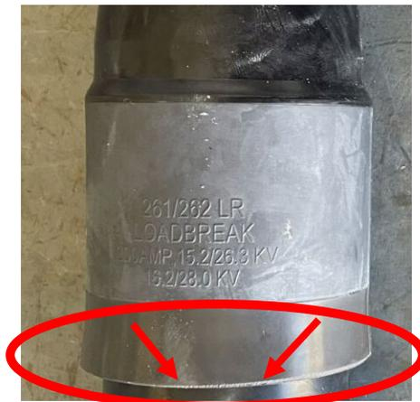
**Figure 2b: Unseated Load Break Elbow**
