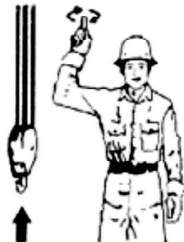
USE MAIN HOIST
