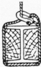
Good Practice— Use space blocks and pad corners
