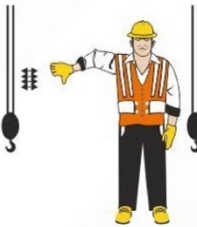
LOWER THE BOOM RAISE THE LOAD
