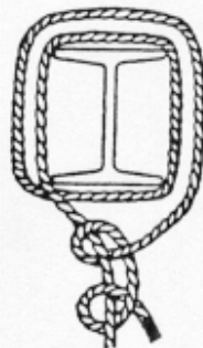
Bad Practice— Steel can cut rope
