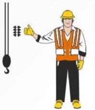
RAISE THE BOOM LOWER THE LOAD
